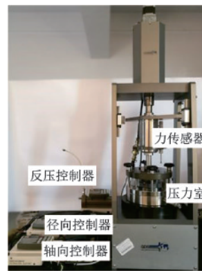
图1 GDS界面剪切试验仪 Fig.1 GDS interface shear apparatus
